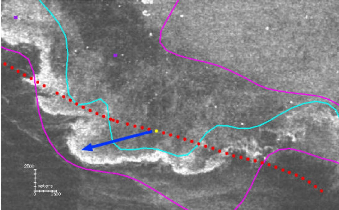
Figure 8. Part of Radarsat image from the 2nd. of July 1999. The drawn ice edge is shown in magenta and the logged position of the aircraft are marked with red dots, one every 10 seconds. The yellow dot and the arrow indicates position and heading of the camera taking the photograph in figure 9.
